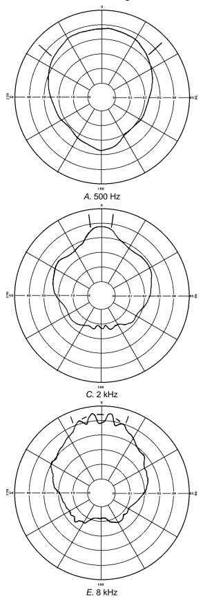
Figure 2. Vertical Polar Plots for Triple-stacked 2370s
