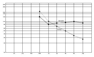
*Figure 4.* Horizontal and Vertical Beamwidth (-6 dB) for a Single 2370
