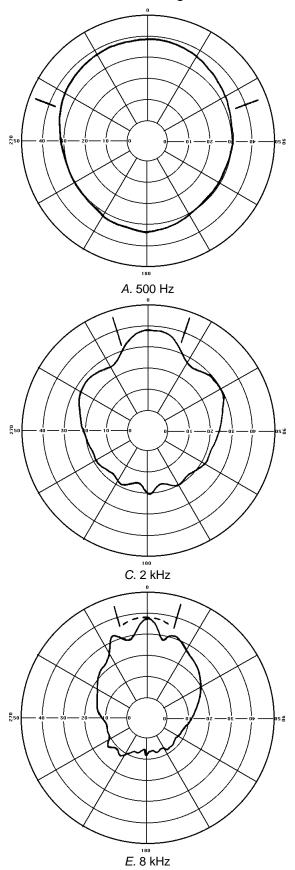
Figure 1. Vertical Polar Plots for Double-stacked 2370s
