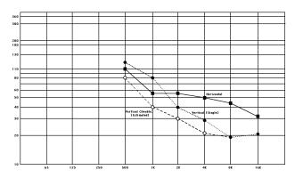
*Figure 9.* Horizontal and Vertical Beamwidth (-6 dB) for a Single 2386 and Double-stacked 2386s
