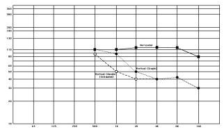
*Figure 7.* Horizontal and Vertical Beamwidth (-6 dB) for a Single 2380 and Double-stacked 2380s
