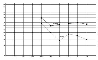
*Figure 6.* Horizontal and Vertical Beamwidth (-6 dB) for a Triple-stacked 2370s
